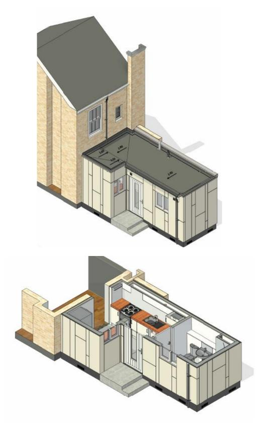
**Figure 50:** 3D view of the proposed extension showing its design and materiality. Refer to the D&A statement (January 2022) for further details of the materials and finishes.
